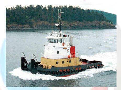
The AluTug Avik Class tug was designed for utilization with barges in the coastwise and river trades of the Pacific Northwest & Alaska. Their stern configuration shrouds the triple screw propellers in tunnels enabling these tugs to work at very shallow drafts. The bow hull form provides seakeeping qualities that allow these tugs to engage in ocean towing.
