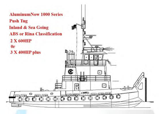
Length:- 23.2m Beam:- 9.77m Depth:- 2.14m Light Draft:- 1.06m Loaded Draft :- 1.47m Classification:- ABS ★ A1 Towing Vessel or as required Construction:- Steel Hull/Aluminium Superstructure Tonnage:- 169 GT – 115 NT – BP(Calculated) 14Tons FWD – 10Tons Astern Towing Wire:- 45m X 32mm wire rope or similar Auxiliary Winches:- Two(2) 60Ton with 30mm wire rope Navigation Equipment:- Radar, GPS, Depthsounder, VHF, Auto-pilot, Sat-com
